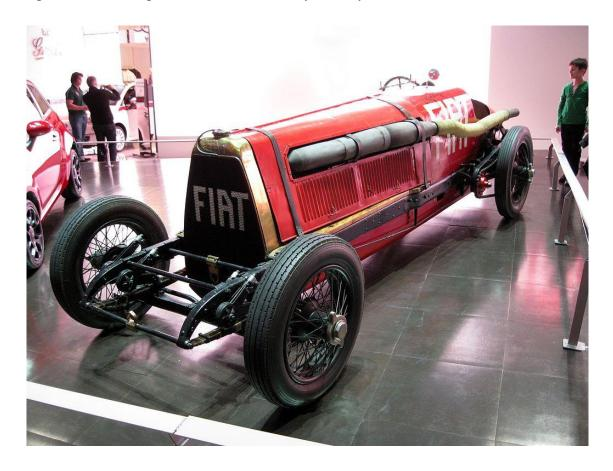
The Fiat Mephistopheles was created by combining the chassis of the 1908 Fiat SB4 with a 6-cylinder, 21.7 litre (21706 cc) Fiat A12 aeroplane engine producing 320 PS (235 kW; 316 bhp). This picture was taken by an unknown photographer at the 2011 Geneva Motor Show. (Another motor show that has disappeared this year. Ed.)
